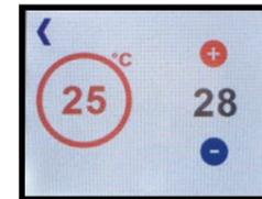
Easy temperature selection with actual cabin temperature (left) and adjustable target temperature (right)
