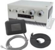
Cabin control kit A-Series<br>Includes: electrical box with controller card, MyTouch display with Webasto cover plate, display cable 5 m, remote air temperature sensor 3 m, max. switching current: 2 x 3.15 A                                                          |                   |                           | ●*                | ●***              | WBCL151000D  |
